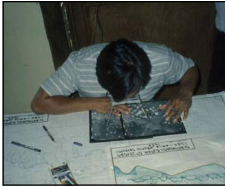
Figure 6.12 Kuna topographer Enrique Arias uses a stereoscope to view 3-D image of the Kuna Yala coastline in aerial photographs supplied by the Instituto Geográfico Nacional. He cross-checks this with a Researcher's sketch map (bottom right) to help locate features on the new map (left).
