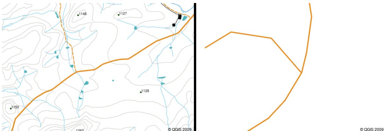
Illustration 19: Polylines viewed at a smaller scale (1:20 000 to the left) may appear smooth and curved. When zoomed in to a larger scale (1:500 to the right) polylines may look very angular.
