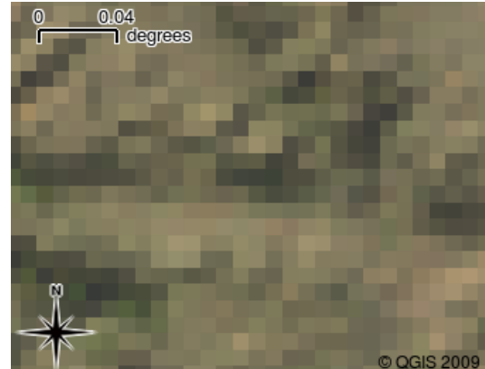
Illustration 13: The same raster data, but this time zoomed in. The grid nature of the data can be seen.
