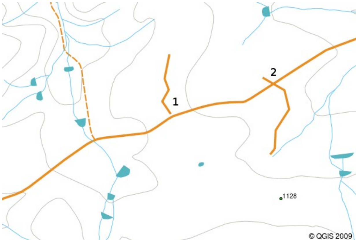
Illustration 26: Undershoots (1) occur when digitised vector lines that should connect to each other don't quite touch. Overshoots (2) happen if a line ends beyond the line it should connect to.
